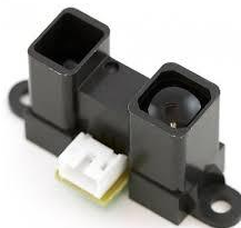
Figure 3. GP2Y0A02YK0F Infra Red Sensor type, Source: https://www.google.co.id/search?q=infrared+tipe+GP2Y0A02YK0F
