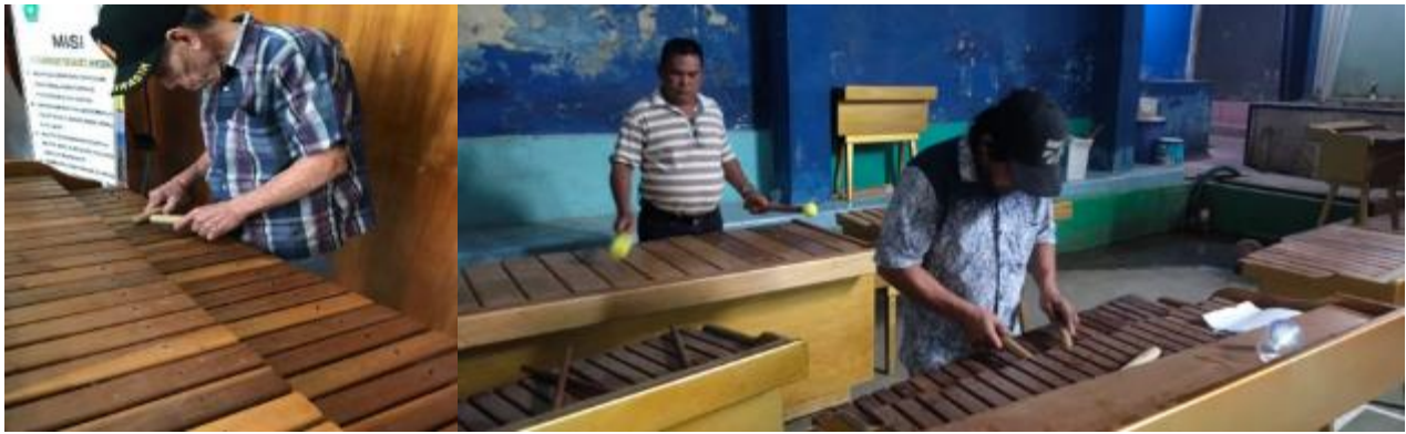
Figure 2. The process of tuning kolintang music to produce the right tone
