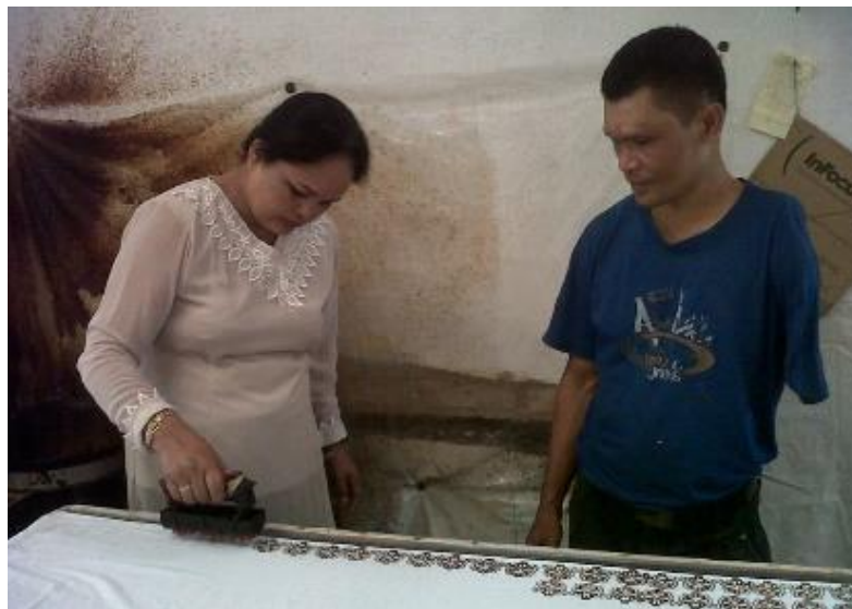
Figure 2. Stamp Batik Making Process (Doc. Isma, 2024)
